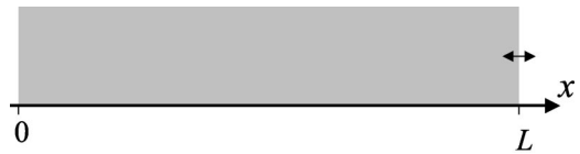
FIG. 2. The rod of a finite length L . The motion of the end at x=L is predetermined by the external loading and is assumed to be known in advance. The end at x=0 is mechanically free.
